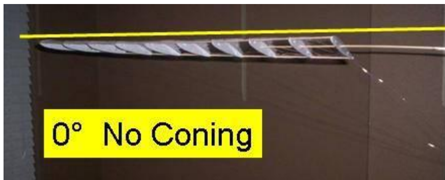
Figure 6-5 Re-rigged Rotor Configuration, in Rotation, No Coning
