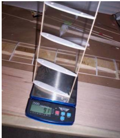
Figure 6-1 Test to Weight the Semi-rigid Rotor
