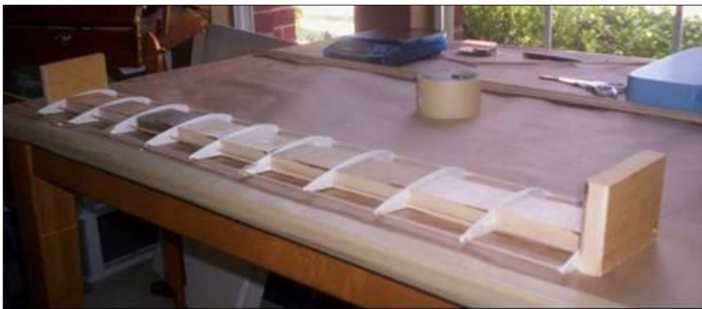
Figure 4-3 Herringbone Fixture: Bonding Ribs and Spars
