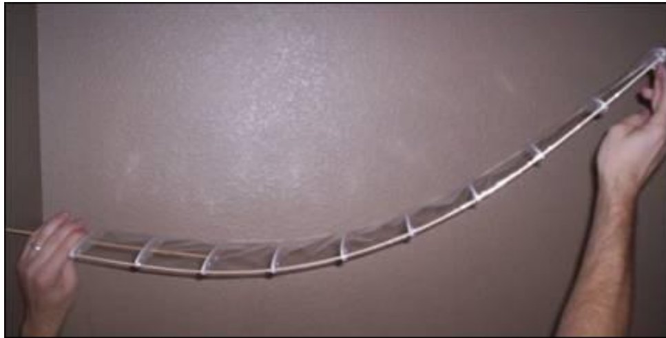
Figure 5-1 Spanwise Bending "Coning" Demo
